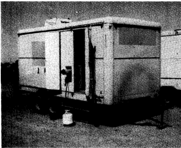
Figure 6a. Self-contained mobile incubator equipped with R-V air conditioner-heater (roof) and outside-venting gas heater for field use.
