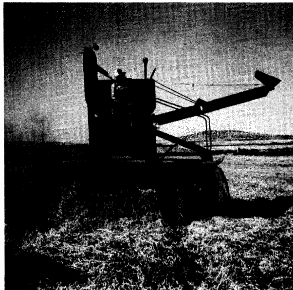
Fig. 5—Self-propelled combine, adapted for alfalfa seed, harvesting seed directly from standing plants after the crop was preconditioned for harvest with a desiccant.
